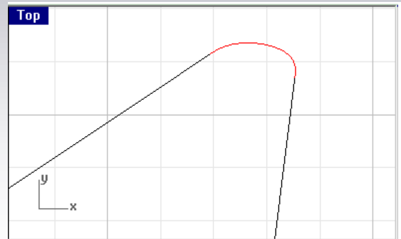
4 curvature continuous blend between curve ends
