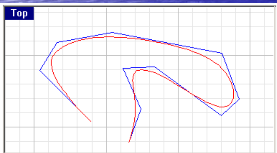
Control point curve through polyline
