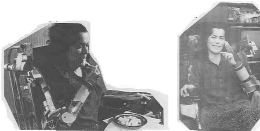
Figure 6. Successfully developed active arm orthosis for rehabilitation of advanced cases of dystrophy and similar diseases. Controlled by means of a joystick. Made in Mihajlo Pupin Institute in 1982.
