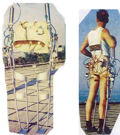
Figure 2. a* and b* First in the world walking active exoskeleton, pneumatically powered and partly kinematically programmed, for producing near-anthropomorphic gait. Made in 1969 at the Mihajlo Pupin Institute, a predecessor of more complex exoskeletons devices for severely handicapped persons.
