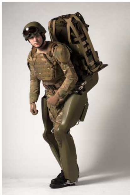
Figure 12. “BLEEX” [8] Project is financed by DARPA It can load up to 32 kg. Man has feeling like 2 kg is on his back. The aim is to improve load up to 60 kg with feeling like 4 kg.
